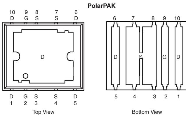
Top surface is connected to pins 1, 5, 6, and 10
