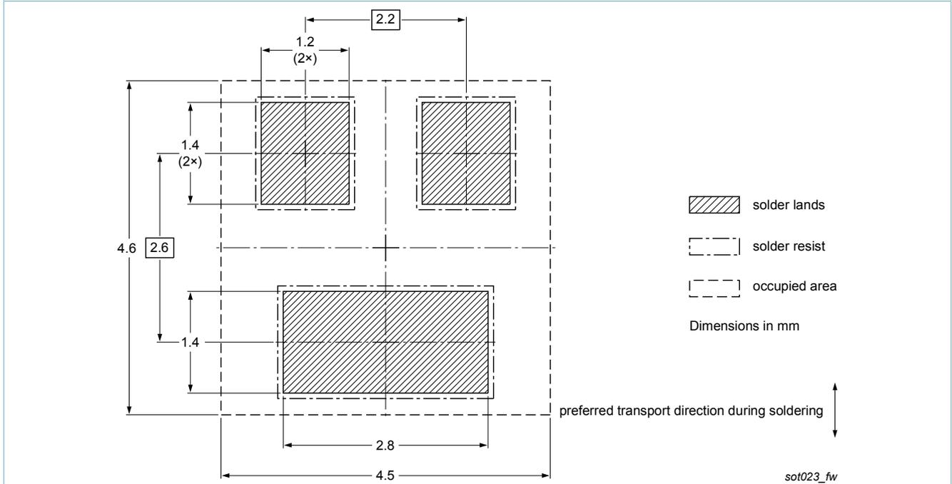
Fig. 20. Wave soldering footprint for TO-236AB (SOT23)
