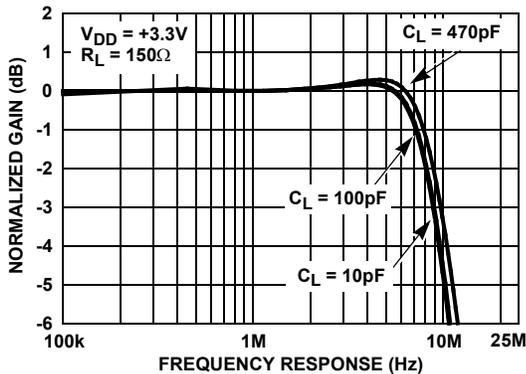
FIGURE 3. GAIN vs FREQUENCY FOR VARIOUS C<sub>LOAD</sub>
