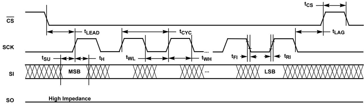
FIGURE 7. INPUT TIMING
