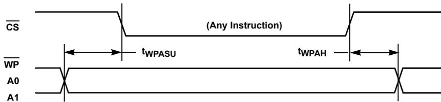
FIGURE 11. WRITE PROTECT AND DEVICE ADDRESS PINS TIMING
