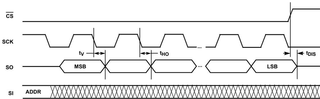
FIGURE 8. OUTPUT TIMING
