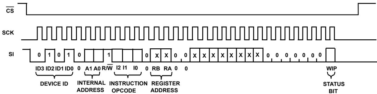
**FIGURE 6. FOUR-BYTE INSTRUCTION SEQUENCE (READ STATUS REGISTERS)**
