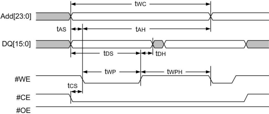
Figure 10-10 Write to Read (tACC) Operation
