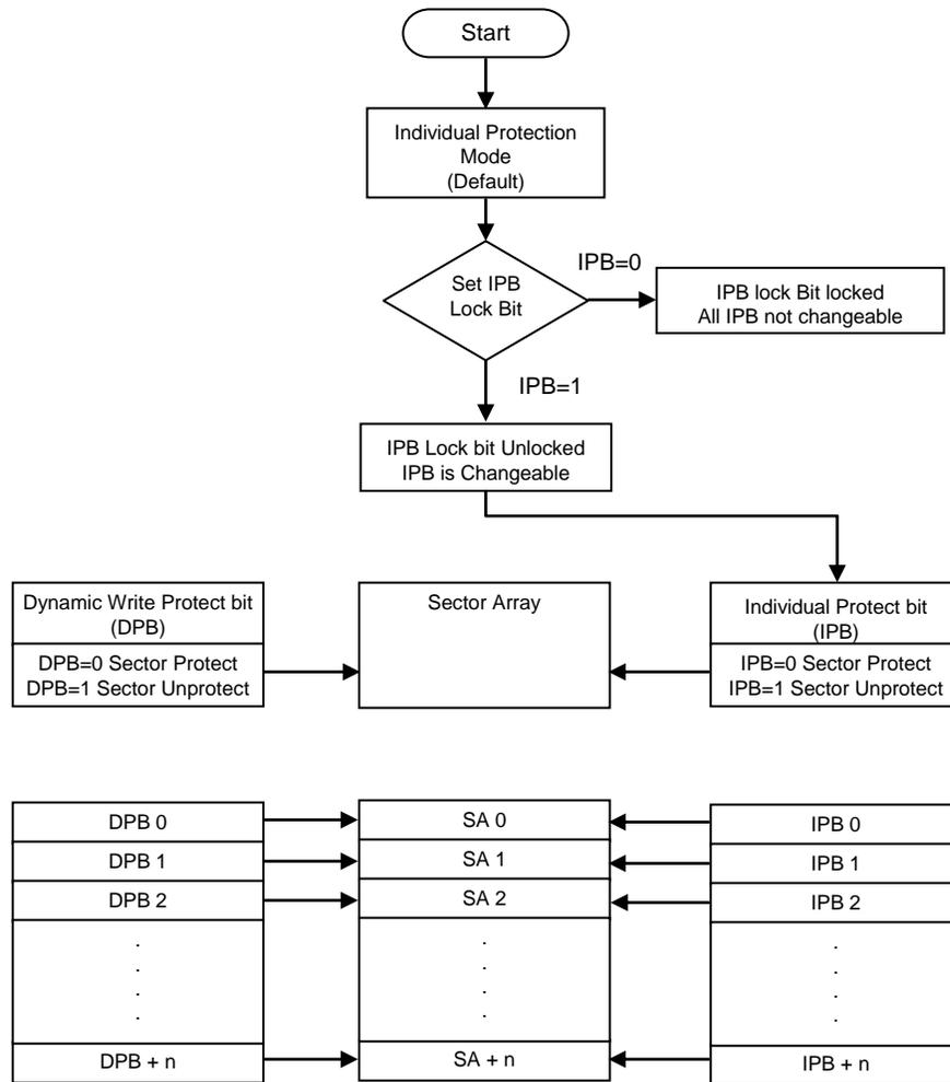
Each sector has a non-volatile Individual Protection Bit (IPB) and a volatile Dynamic Protection Bit (DPB) associated with it. If in either case the bit is 0, the sector becomes protected from both program and erase operations.
