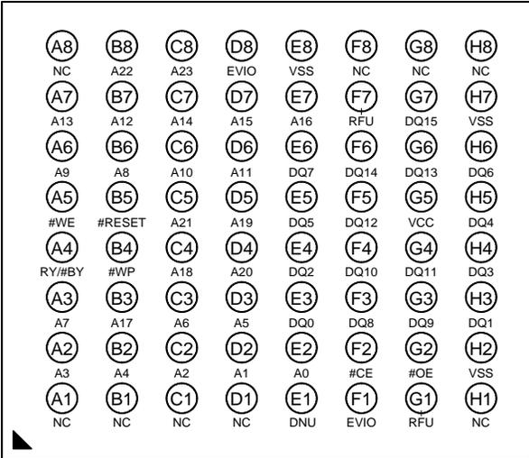
Figure 3-2 56-PIN STANDARD TSOP (Top View)
