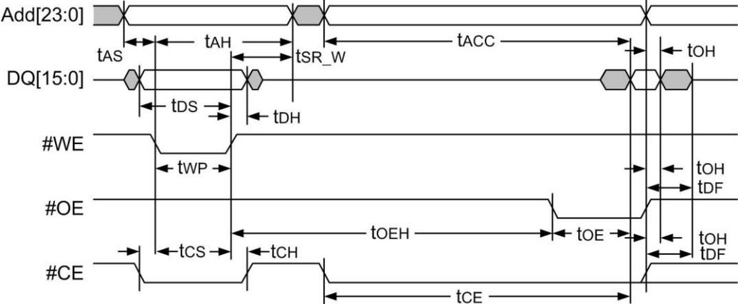
Figure 10-12 Read to Write (#CE VIL) Operation
