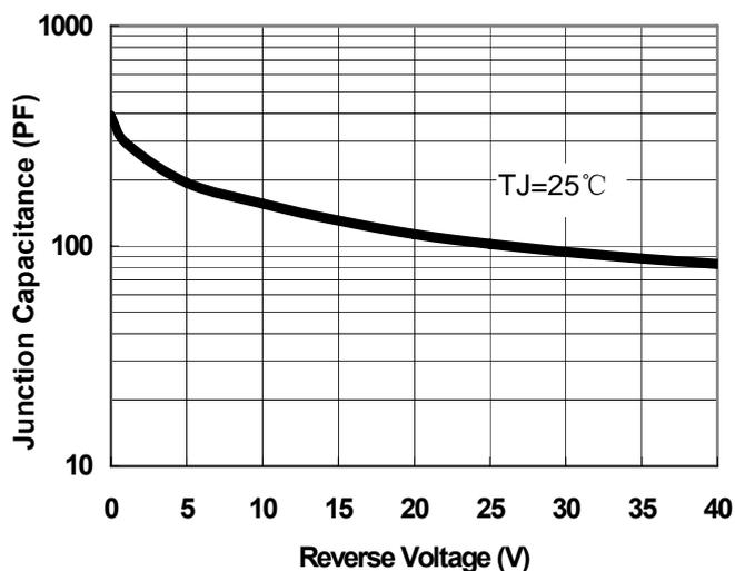
Fig.1-Typical Junction Capacitance
