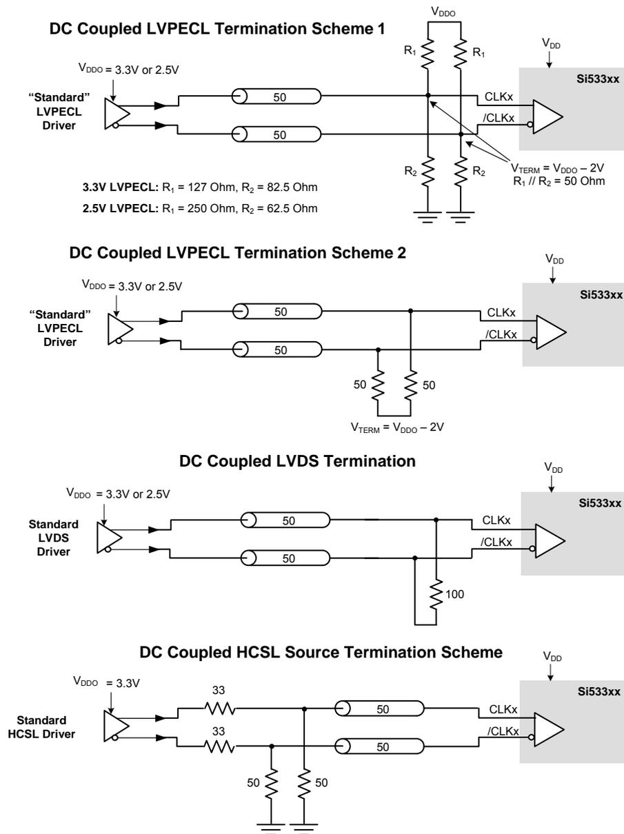
Note: 33 Ohm series termination is optional depending on the location of the receiver.
