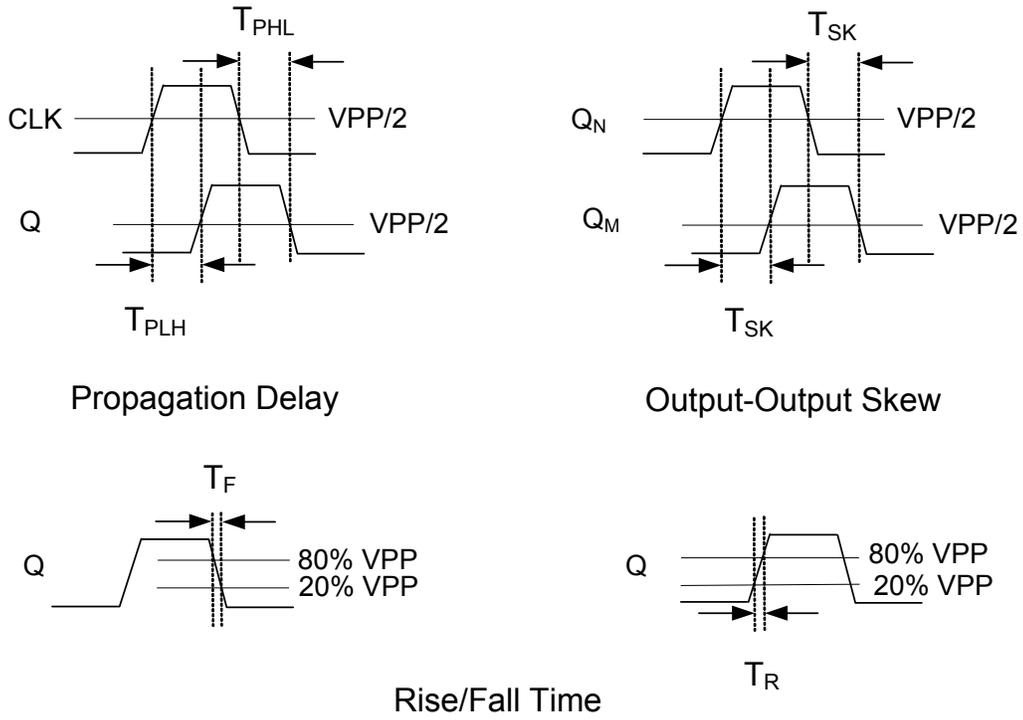
Figure 12. AC Waveforms
