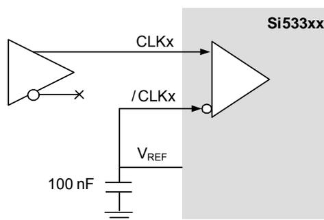
**Figure 6. Using Voltage Reference with Single-Ended Input Clock**
