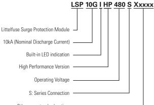
Other non-standard option: **X3333:** with GND wire connection, available at a 277Vac rating CE marked, for Class I installations, earthed.
