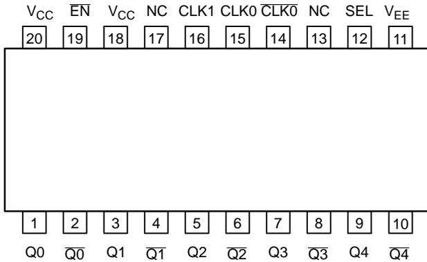
Note: All V<sub>CC</sub> and V<sub>EE</sub> pins must be externally connected to Power Supply to guarantee proper operation.
