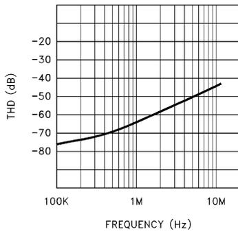
FIGURE 5. DISTORTION vs FREQUENCY
