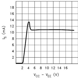
FIGURE 1. I<sub>S</sub> vs SUPPLY VOLTAGE
