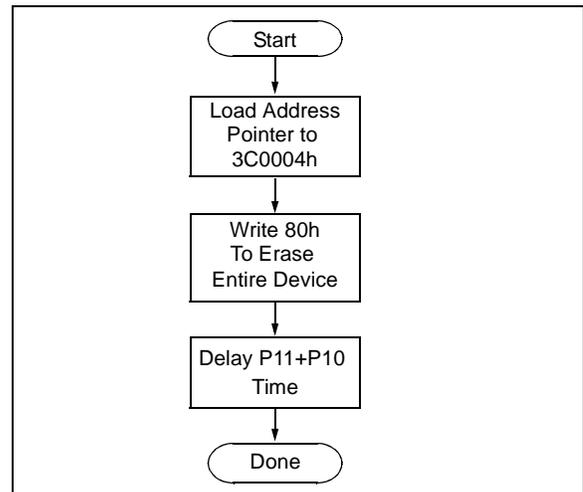
**FIGURE 3-3: BULK ERASE TIMING**
