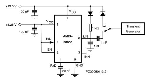
Figure 7. Test Circuit for Transient Measurements
