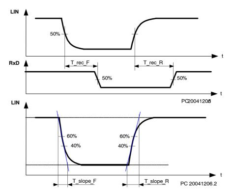
Figure 5. Timing Diagram for AC Characteristics According to LIN 1.3
