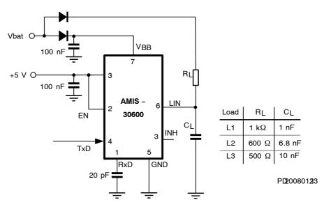
Figure 4. Test Circuit for Timing Characteristics
