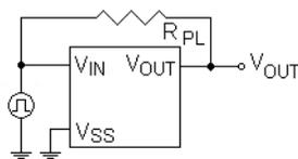
Pull-up Resistor  $R_{PL} = 100\text{ k}\Omega$  is used for IXD5120N version only
