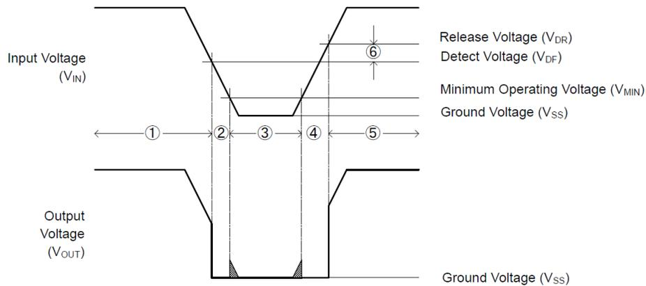
Note: To simplify explanation, an operation time of the circuit is not included.
