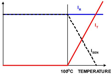
FIGURE 7. CURRENT SIGNALS AT THE AMPLIFIER CA INPUT.
