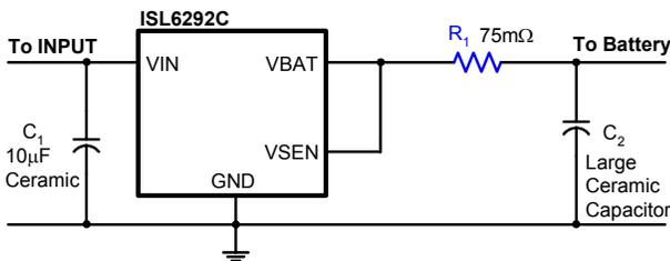
**FIGURE 9. INSERTING R<sub>1</sub> TO IMPROVE THE STABILITY OF APPLICATIONS WITH LARGE CERAMIC CAPACITOR IS USED AT THE OUTPUT**
