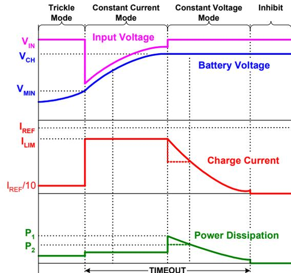
FIGURE 4. TYPICAL CHARGE CURVES USING A CURRENT-LIMITED ADAPTER
