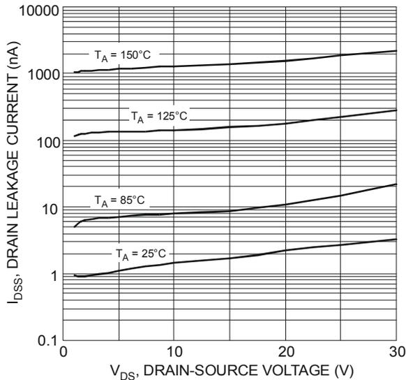
Figure 9 Typical Drain-Source Leakage Current vs. Voltage
