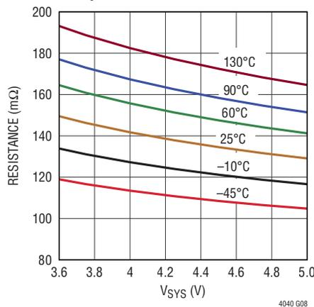
**Step-Down Charger NMOS On-Resistance vs  $V_{SYS}$  over Temperature**
