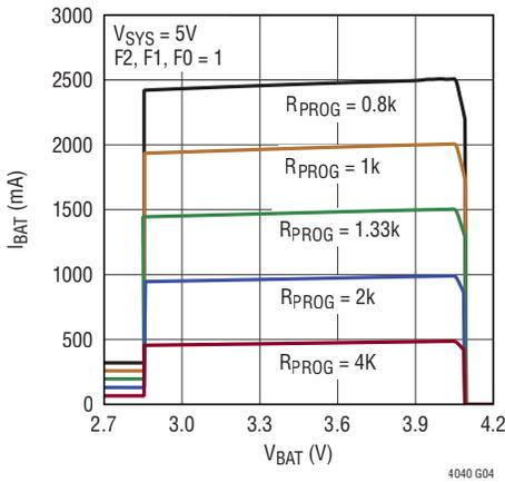
**$I_{BAT}$  vs  $V_{BAT}$  (LiFePO<sub>4</sub>) with Different PROG Resistor Values**
