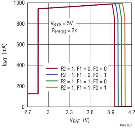
**$I_{BAT}$  vs  $V_{BAT}$  (LiFePO<sub>4</sub>) with Different Charge Voltage Settings**
