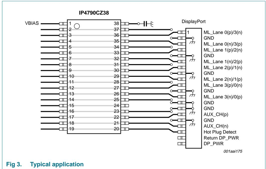
Connecting an optional 100 nF capacitor to the BIAS\_CAP pin (lead 38) enhances the ESD protection clamping performance. The VBIAS pin reduces the capacitive load of the ESD protection and  $V_{VBIAS}$  can be in the range 2.5 V to 5.5 V.
