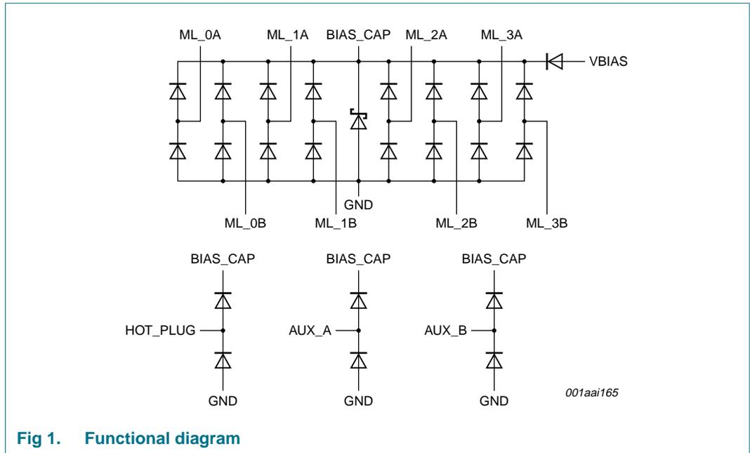
Fig 1. Functional diagram
