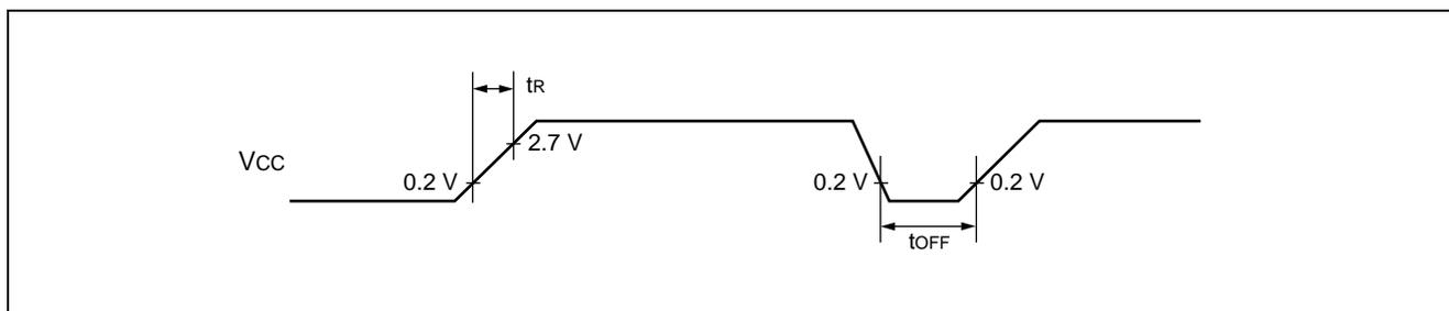
Note : Sudden change of power supply voltage may activate the power-on reset function. When changing power supply voltages during operation, raise the power smoothly by suppressing variation of voltages as shown below. When raising the power, do not use PLL clock. However, if voltage drop is 1V/s or less, use of PLL clock is allowed during operation.
