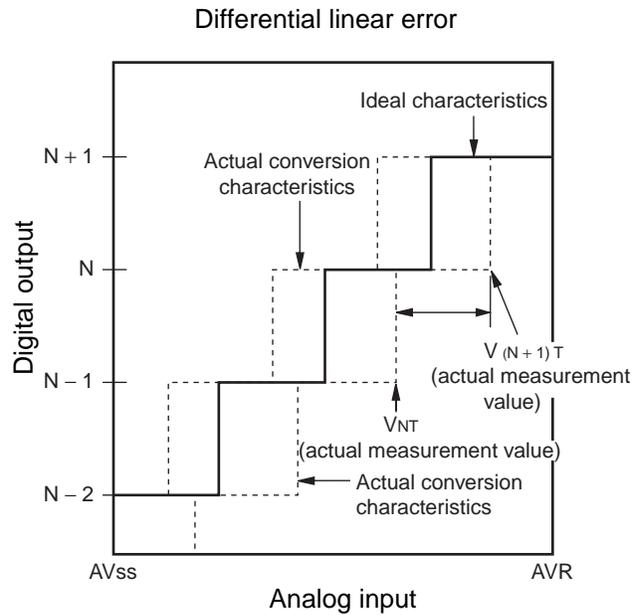
$$\text{Linear error of digital output } N = \frac{V_{NT} - \{1 \text{ LSB} \times (N - 1) + V_{OT}\}}{1 \text{ LSB}} \text{ [LSB]}$$
