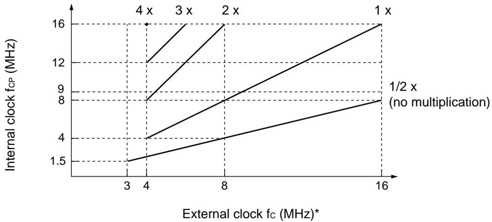
\* :  $f_c$  is 8 MHz at maximum when crystal or ceramic resonator circuit is used.
