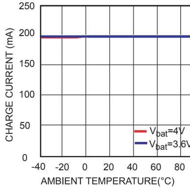
**Charge Current(500mA) vs. Ambient Temperature**
