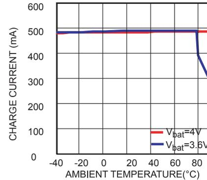
**Charge Current(800mA) vs. Ambient Temperature**
