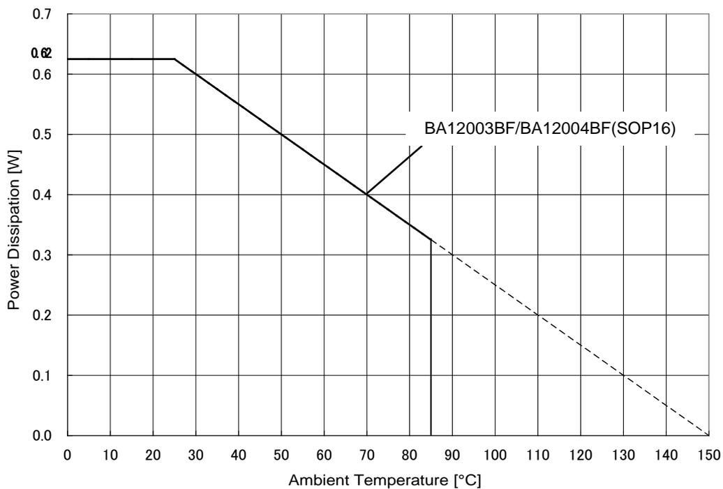
Figure 17. Derating curve
