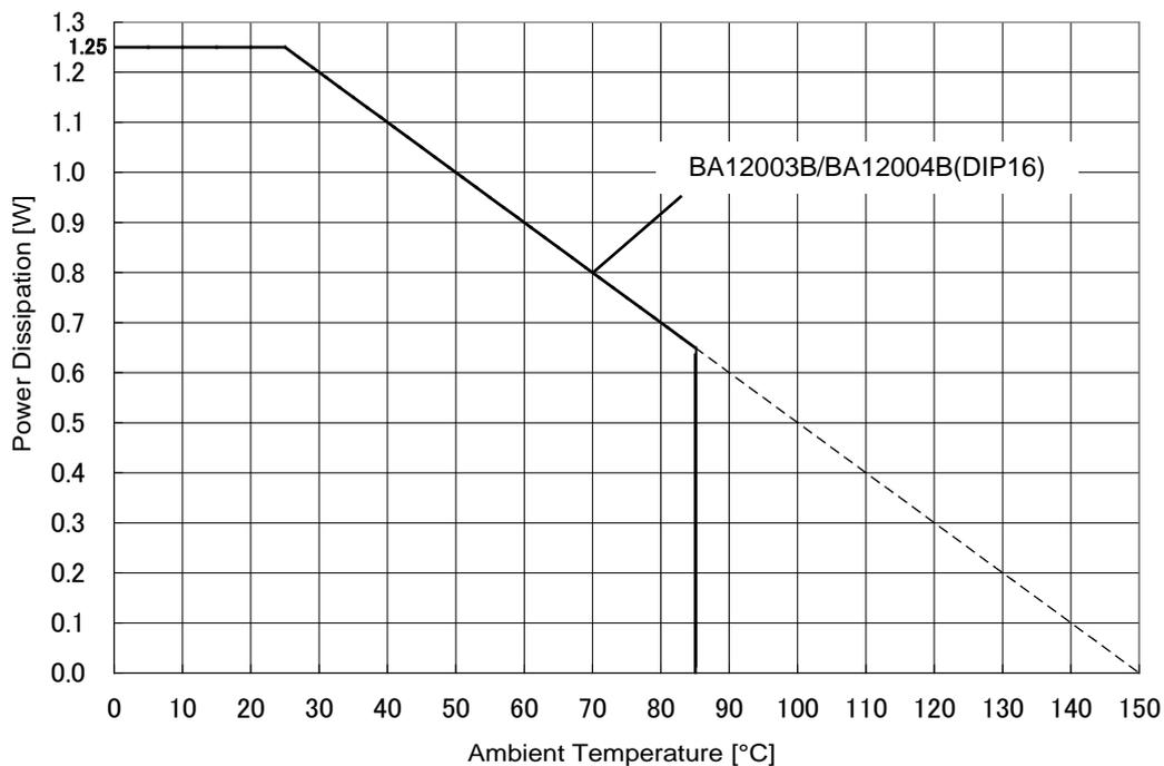
Figure 16. Derating curve
