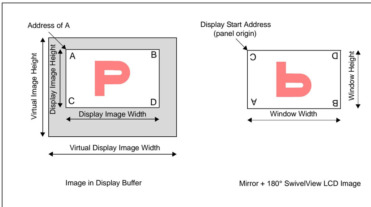
Figure 13-4: Mirror Display with 180° SwivelView Display
