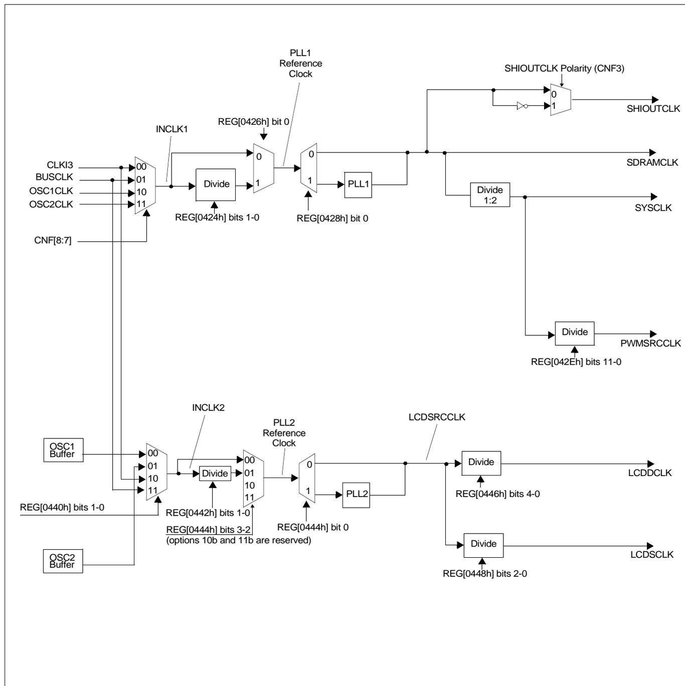
Figure 9-1: Clock Diagram
