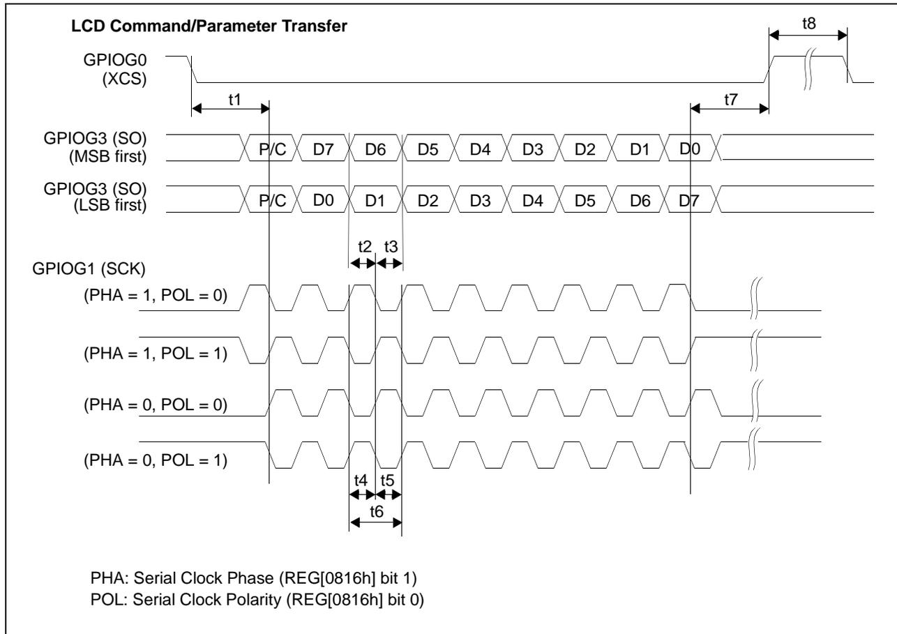
Figure 7-20: ND-TFD 9-Bit Serial Interface Timing
