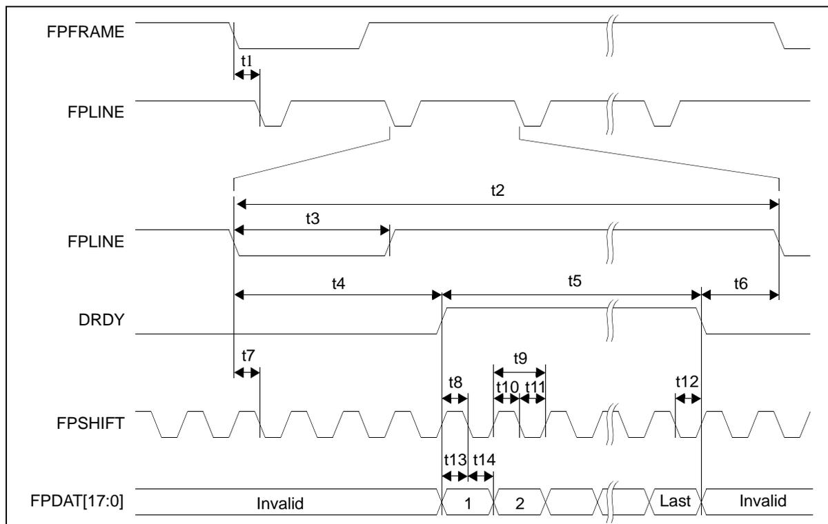
Figure 7-17: Generic RGB Type Interface Panel Horizontal Timing
