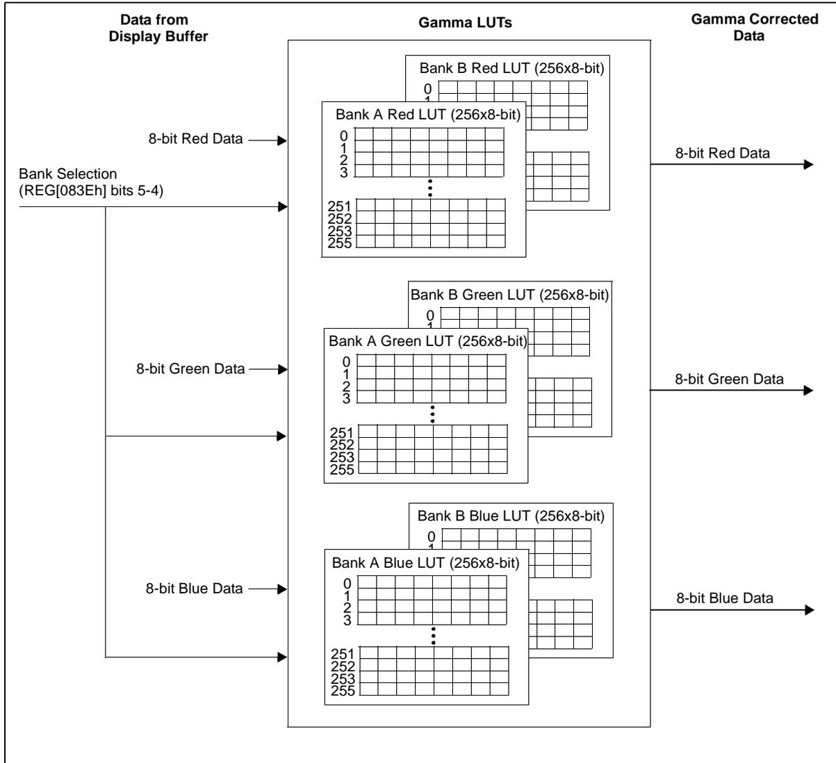
Figure 13-5: Gamma LUT Architecture for Color Modes
