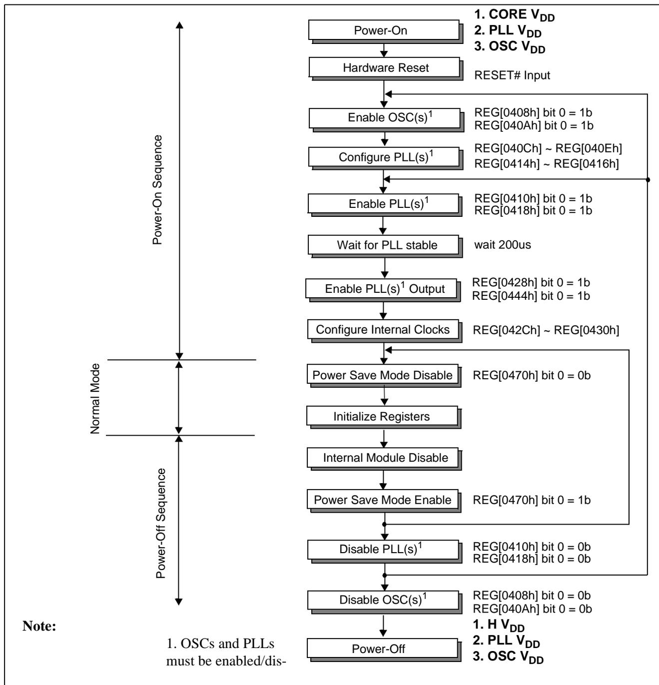
Figure 11-1: Power-On/Power-Off Sequence
