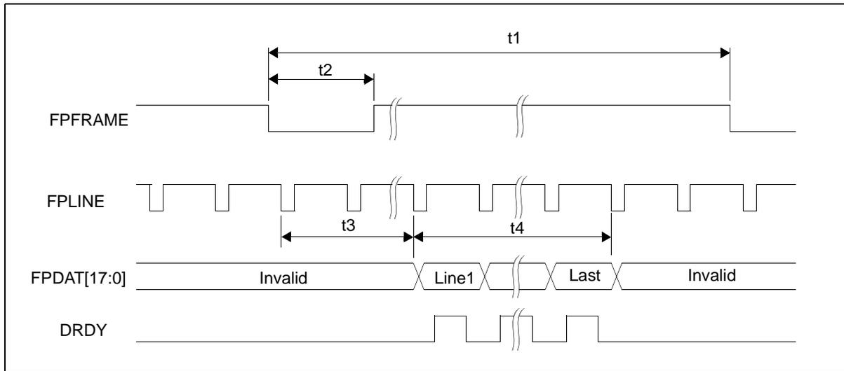
Figure 7-18: Generic RGB Type Interface Panel Vertical timing
