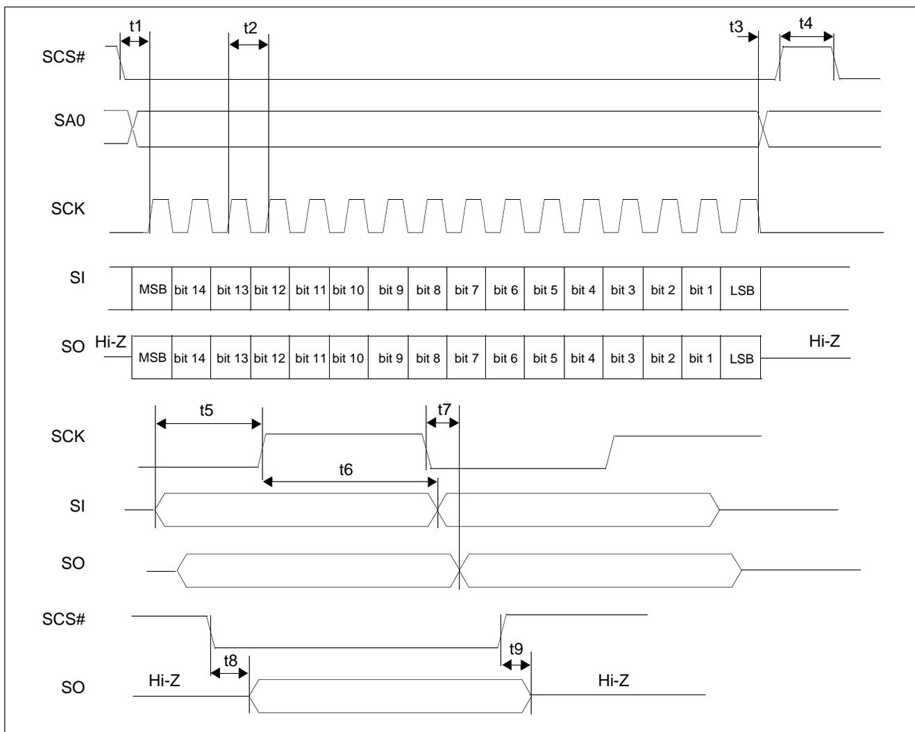
Figure 7-13: Serial Host Interface Timing for Data Valid on Falling Edge of SCK
