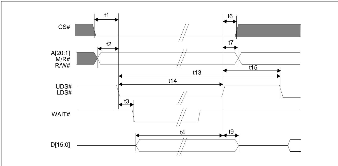
Figure 7-11: Direct/Indirect 68 Host Interface Write Timing
