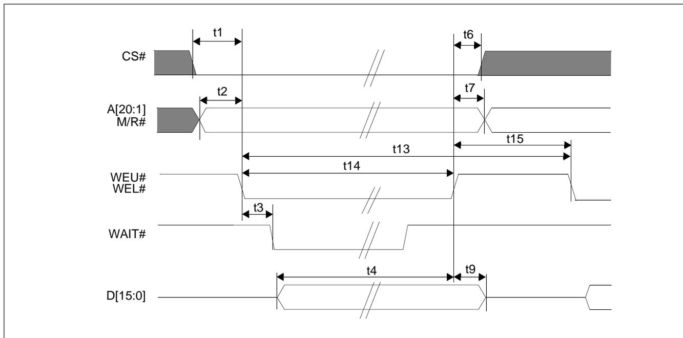
Figure 7-9: Direct/Indirect 80 Type 2 Host Interface Write Timing
