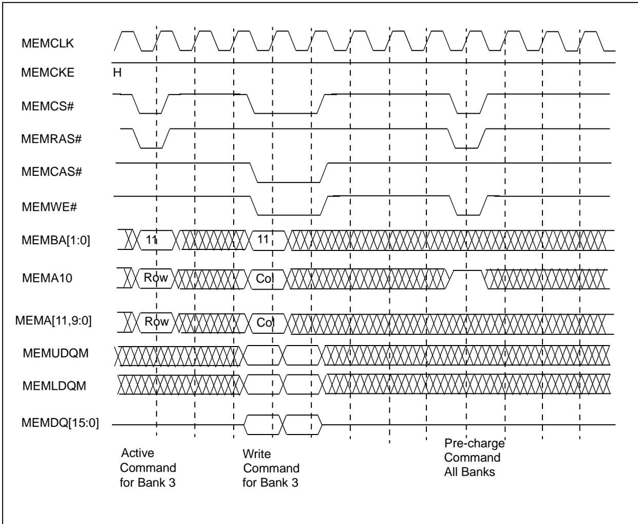
Figure 7-26: SDRAM Write Timing (Ex. Write Length = 2)
