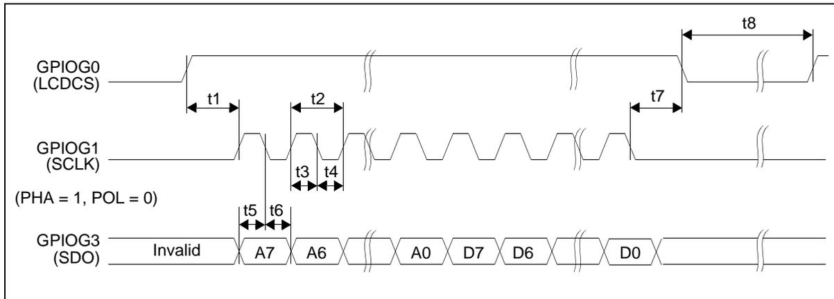
Figure 7-22: uWIRE Serial Interface Timing
