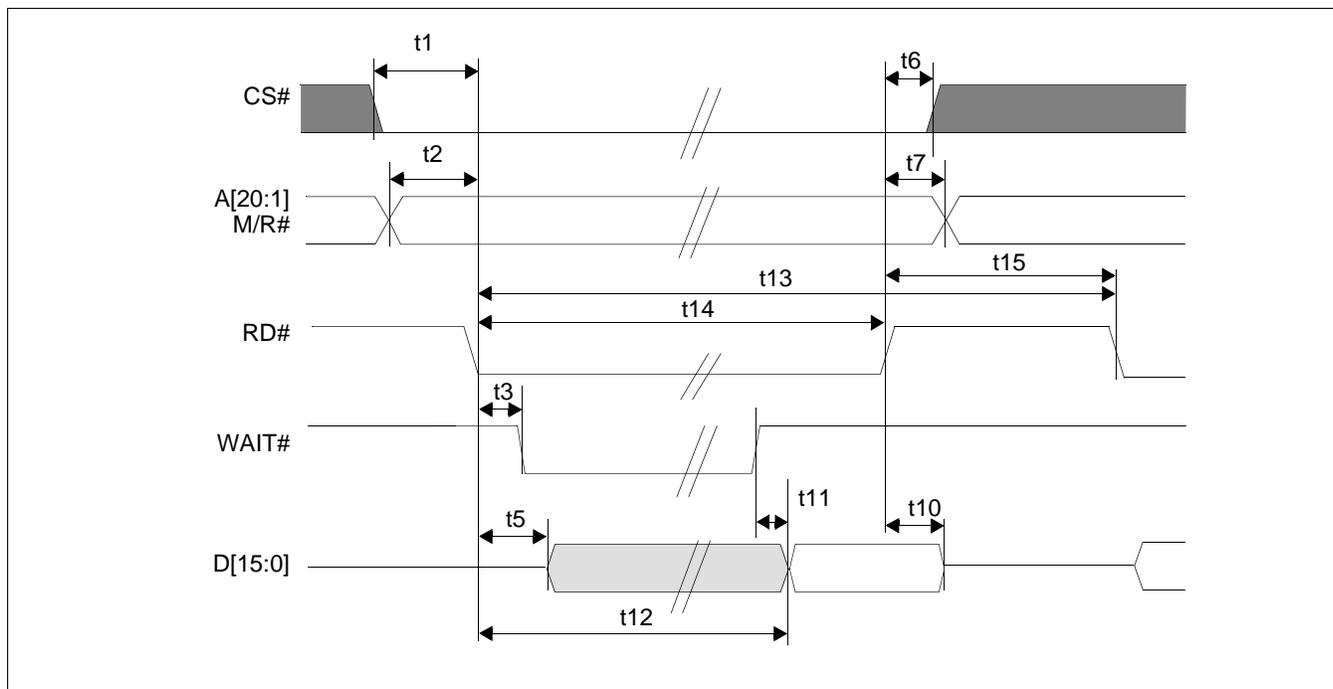
Figure 7-10: Direct/Indirect 80 Type 2 Host Interface Read Timing
