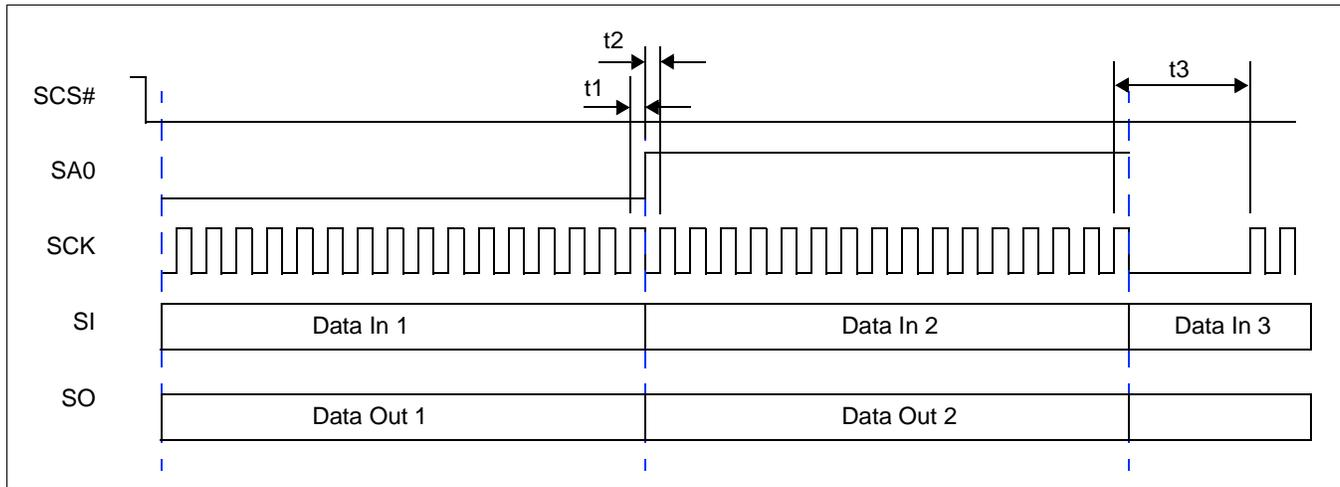
Figure 7-15: Serial Host Interface Burst Mode Timing
