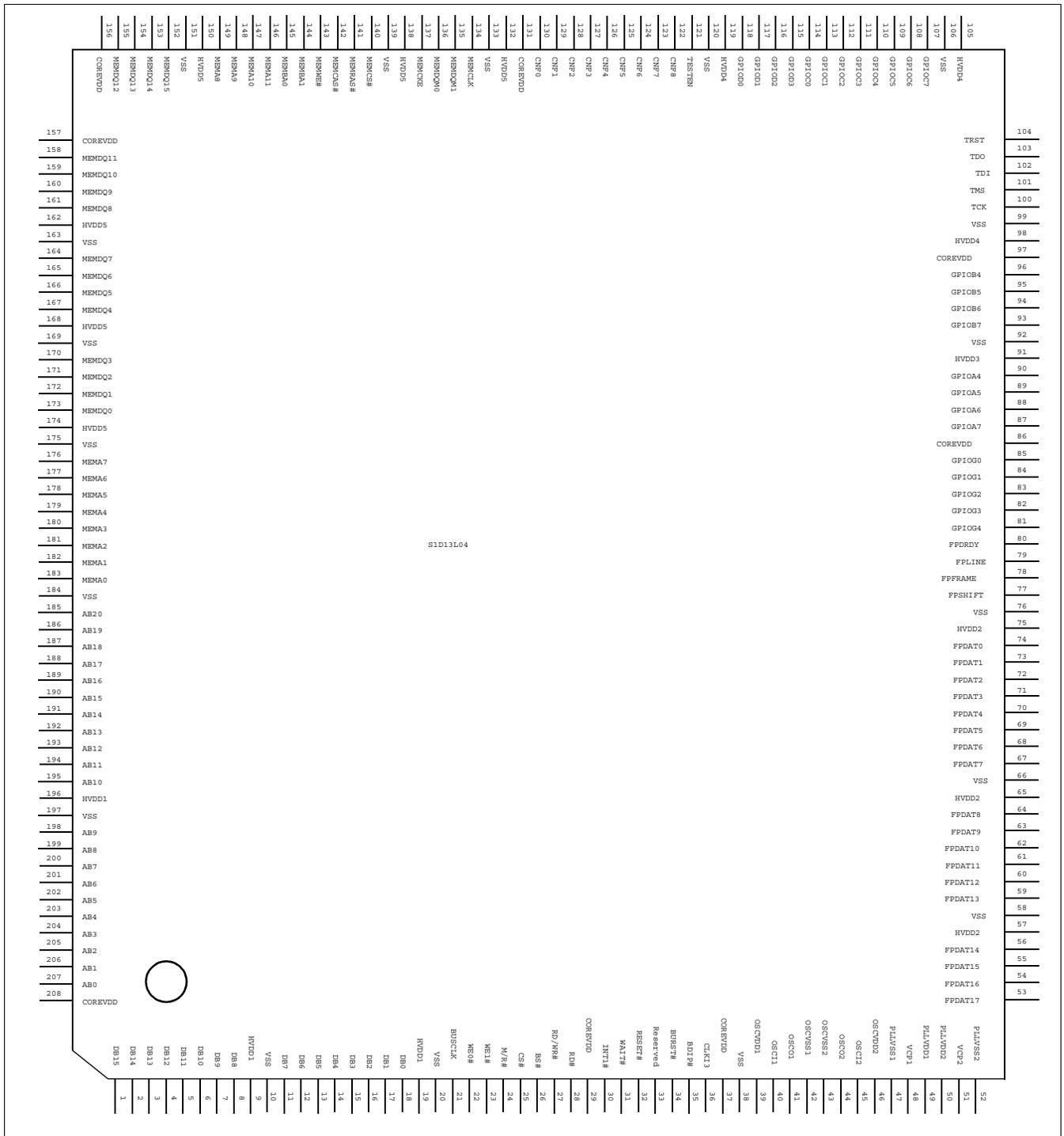
Figure 5-1: QFP22-208 Pinout
