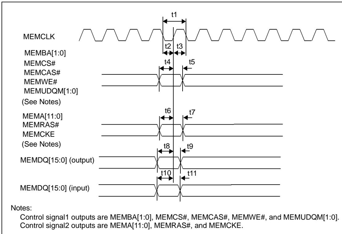
Figure 7-24: SDRAM Setup/Hold to MEMCLK Timing
