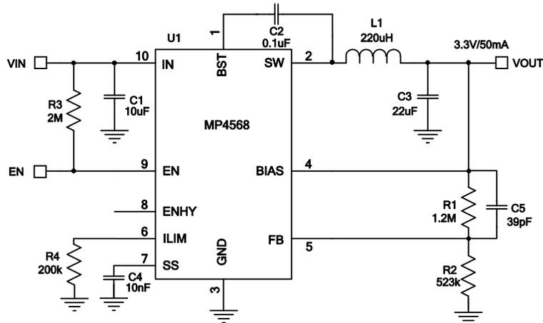
Figure 10 – 3.3V/50mA Output Typical Application Circuit
