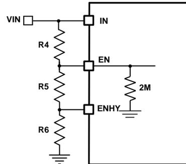
**Figure 6 – Adjustable UVLO using EN & ENHY pin**
