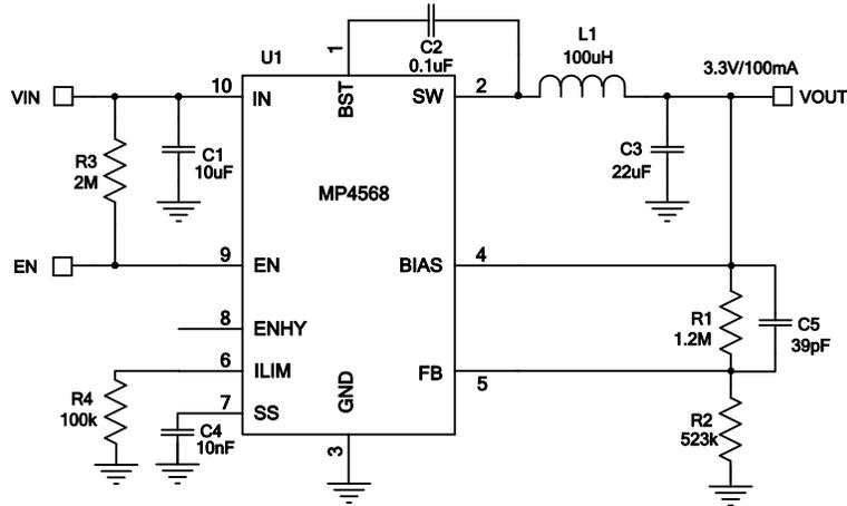
Figure 9 – 3.3V/100mA Output Typical Application Circuit
