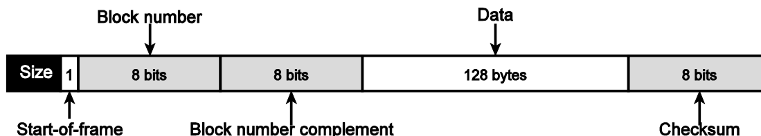
Figure 2-9. X-Modem Frame Structure
