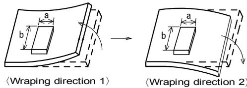
Products(A,B,C,D) shall be located carefully so that products are not subject to the mechanical stress due to warping the board. Because they may be subjected the mechanical stress in order of  $A \cdot C > B \cong D$ .
