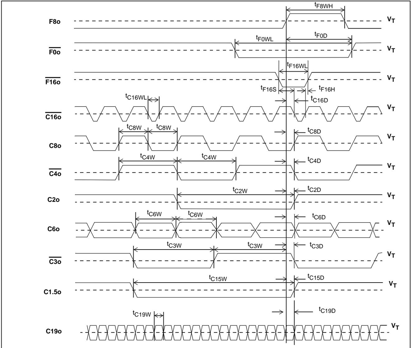
Figure 20 - Output Timing 1
