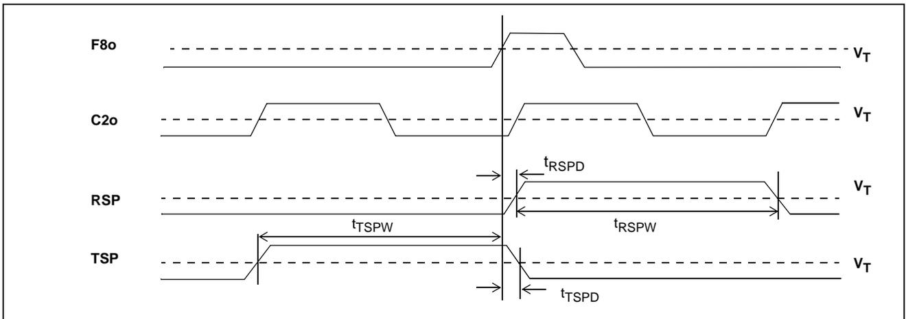
Figure 21 - Output Timing 2
