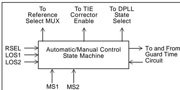
**Figure 6 - Automatic/Manual Control State Machine Block Diagram**
