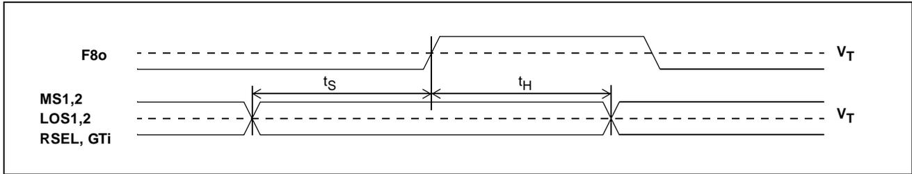
Figure 22 - Input Controls Setup and Hold Timing
