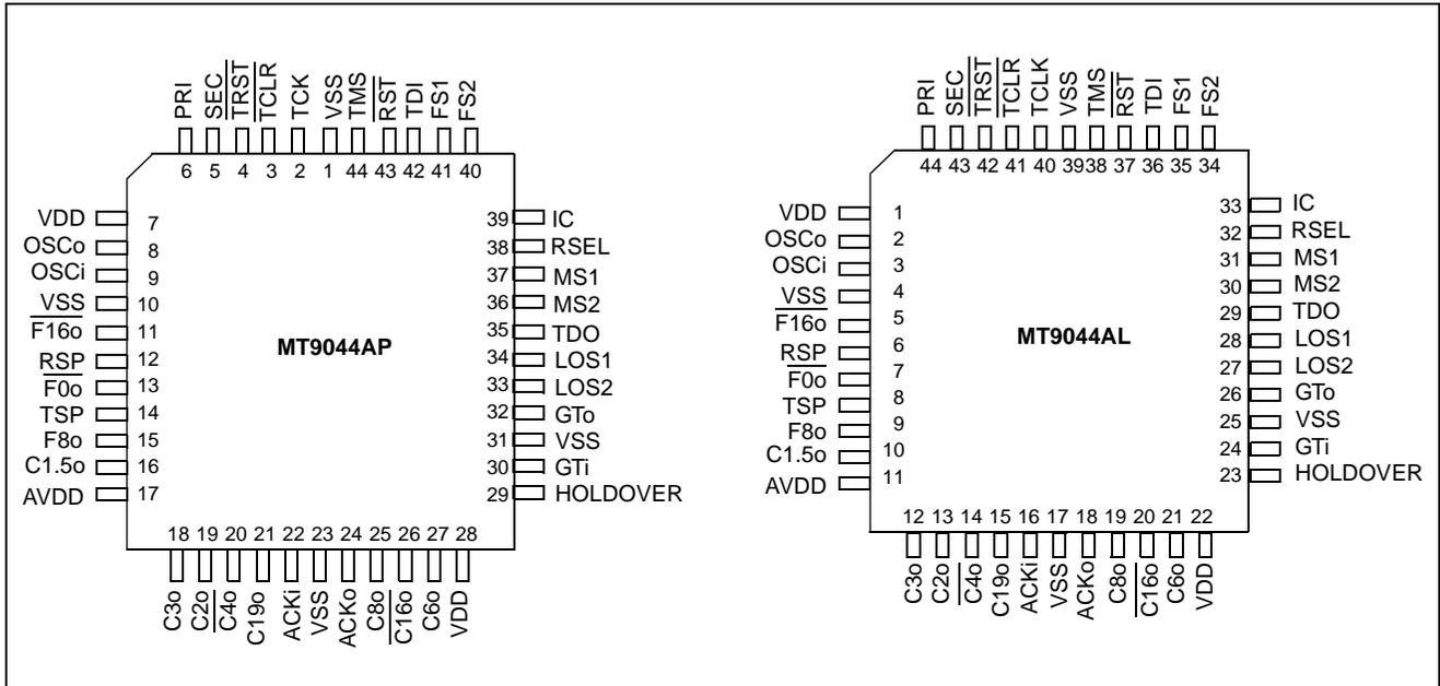
**Figure 2 - Pin Connections**
