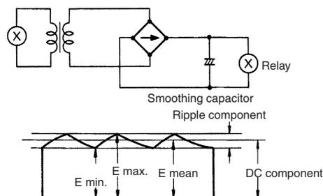
$$\text{Ripple percentage} = \frac{E_{\text{max.}} - E_{\text{min.}}}{E_{\text{mean}}} \times 100$$
