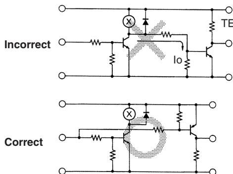
A circuit that produces a control output as soon as the relay operates must be carefully designed. In the first example, electrode dark current flows as shown when the relay operates. When dark current flows into the relay coil, the relay's resistivity to shock and vibration may degrade.
