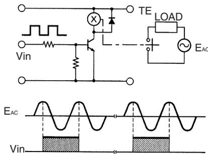
If the relay operates in synchronization with the supply voltage, the life of the relay may be shortened. When designing the control system in which the relay is used, estimate the life of the relay and thus the reliability of the overall system under actual operating conditions. Moreover, construct the circuit so that the relay operates in a random phase or in the vicinity of the zero point.
