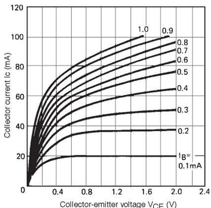
7. Using the following formula, calculate the power dissipated by the transistor to confirm that it is within the range of permissible power dissipation of the transistor.
