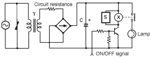
If a load such as a capacitor or lamp through which an inrush current flows is connected to the power source and contact of the relay, the supply voltage may drop when the contact is closed, causing the relay to abnormally release.
