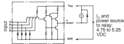
2. To drive a relay with open-collector output type TTL, a degree of freedom is allowed in the ratings of the relay coil. However, these conditions must be satisfied:
