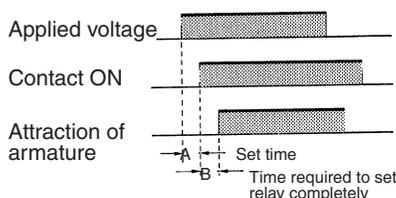
Therefore, it is apparent that time constant T obtained as the product of C and R must be equal to or longer than the sum of A and B. Actually, however, T should not be equal to the sum of A and B but must be longer than that to ensure the stable operation of the circuit. Thus,  $T = A + B + X$
