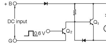
The TTL output of a solid-state switch can be used as Q<sub>2</sub>.
