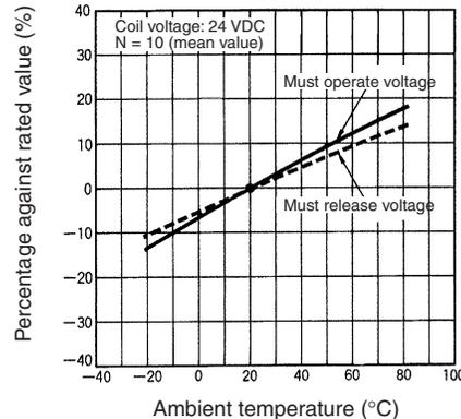
The minimum must operate voltage can be determined by this expression.
