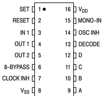
Figure 1. Pin Assignment
