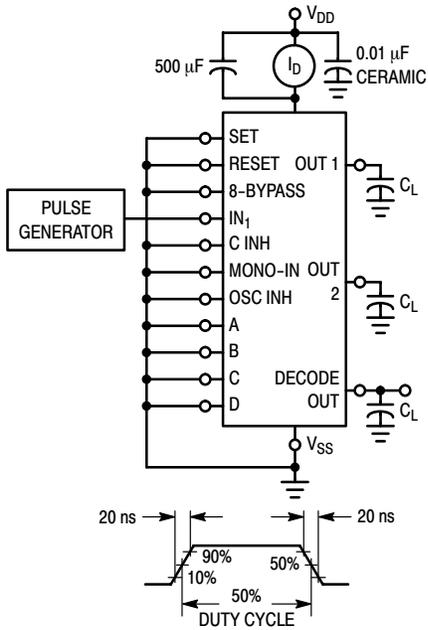
**Figure 8. Power Dissipation Test Circuit and Waveform**
