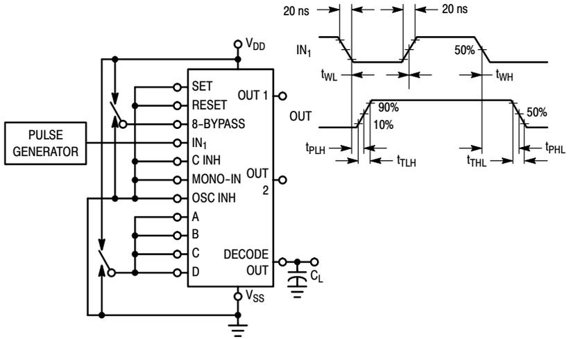
**Figure 9. Switching Time Test Circuit and Waveforms**
