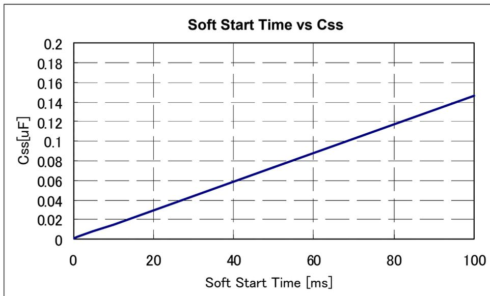
Figure : Soft Start Time vs C<sub>SS</sub> Value ( External Capacitor )
