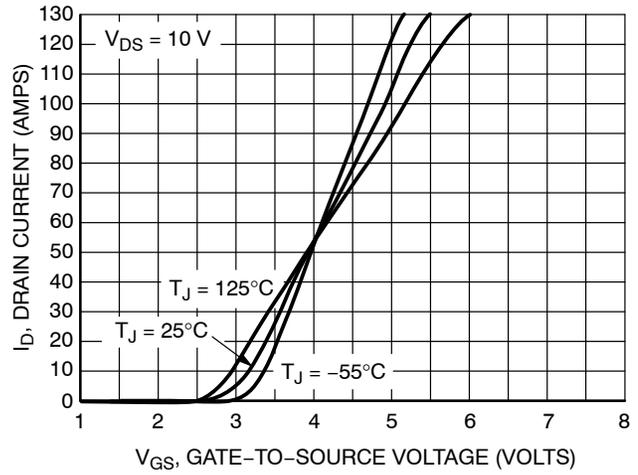
Figure 2. Transfer Characteristics
