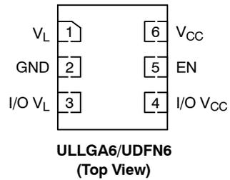
Figure 6. Pin Assignments
