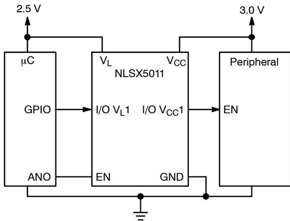
Figure 3. Application Example for  $V_L < V_{CC}$
