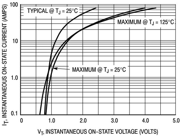
Figure 3. On-State Characteristics
