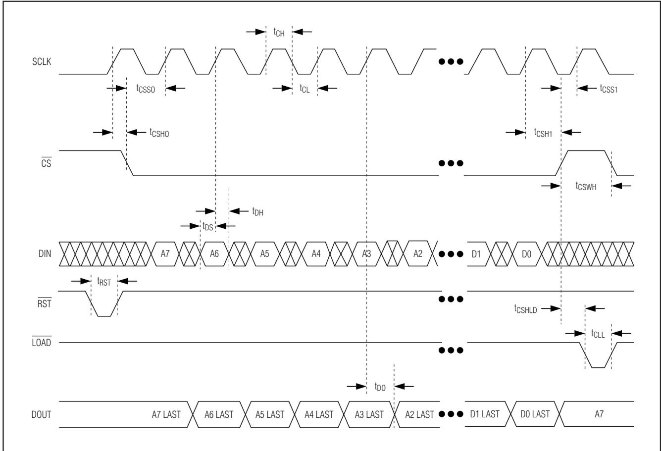
Figure 9. Serial-Interface Timing
