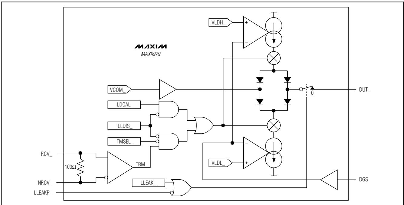
Figure 5. Active Load Block Diagram (One Channel Shown)
