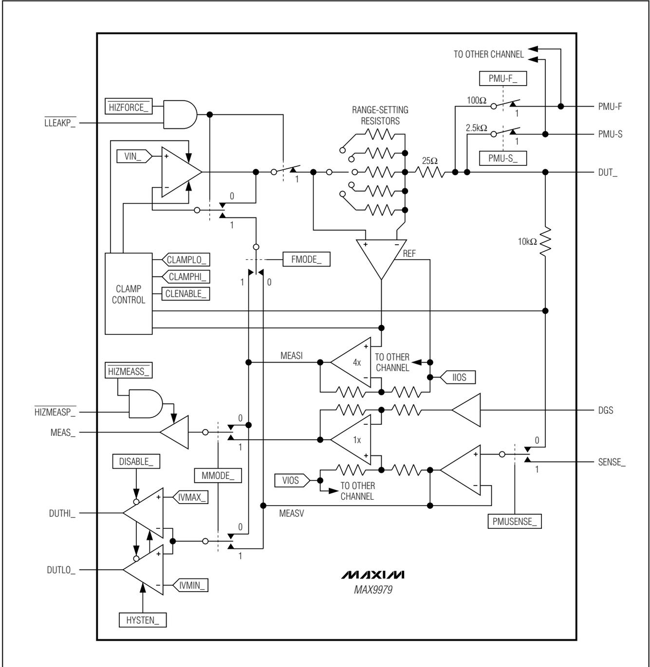
Figure 6. PMU Block Diagram (One Channel Shown)
