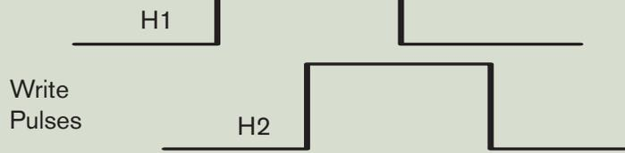
Figure 5. The current pulse sequence used to produce the sequence of magnetic fields used for toggle switching.
