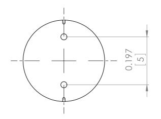
\*For 220µH and up, diameter = 0.354/9.0 Max \*\*\* Optional lead length: L: 0.67/17, P: 0.39/10
