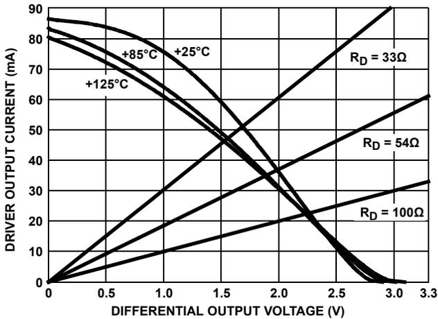
FIGURE 10. DRIVER OUTPUT CURRENT vs DIFFERENTIAL OUTPUT VOLTAGE
