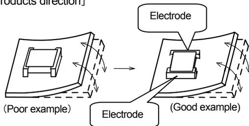
Products shall be located in the sideways direction to the mechanical stress.
