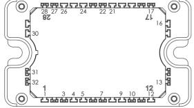
All multiple inputs and outputs must be shorted together Example: 10/11; 13/14; 6/7...
