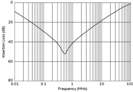
Common Mode Insertion Loss (Typ.)
