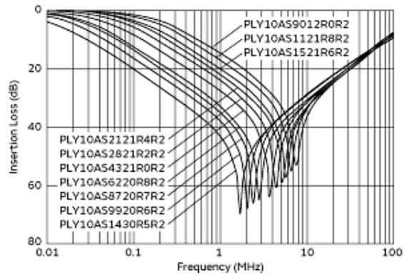
Differential Mode Insertion Loss-Frequency Characteristics
