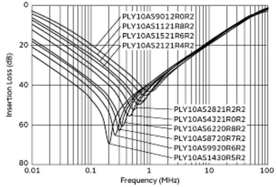
Common Mode Insertion Loss-Frequency Characteristics
