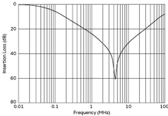
Differential Mode Insertion Loss (Typ.)
