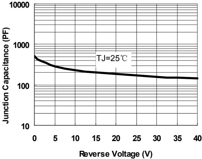
Fig.1-Typical Junction Capacitance
