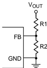
Figure 1. Setting V<sub>OUT</sub> with a Voltage Divider
