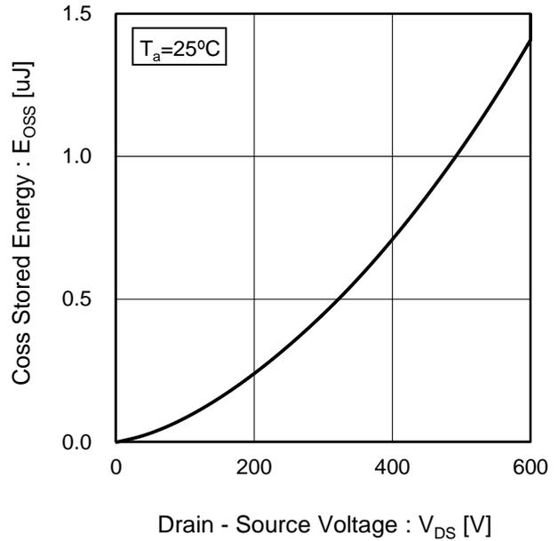
Fig.20 Switching Characteristics
