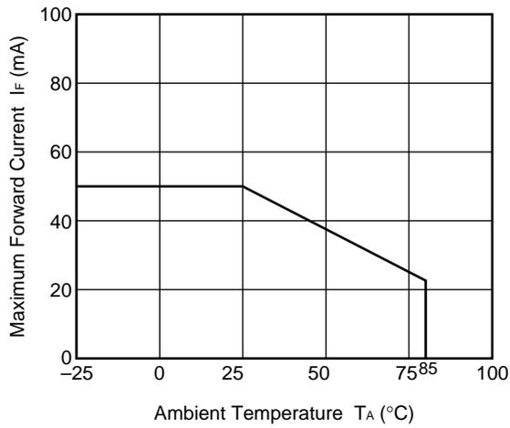
MAXIMUM LOAD CURRENT vs. AMBIENT TEMPERATURE
