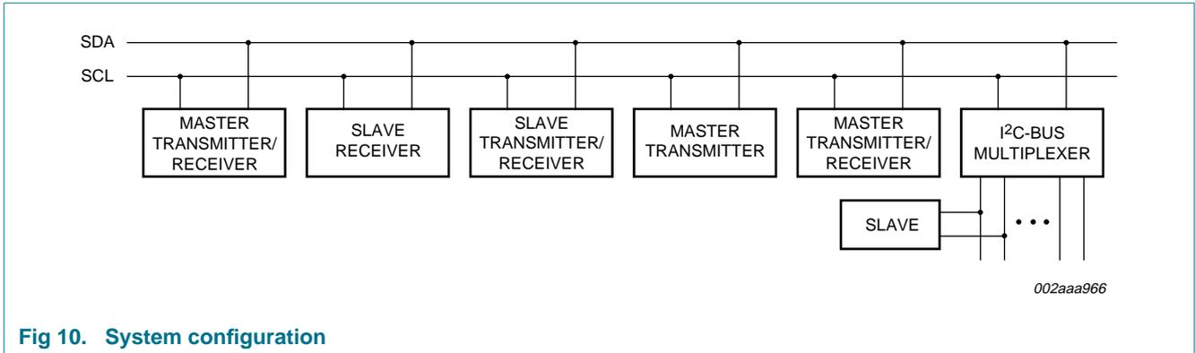
Fig 10. System configuration
