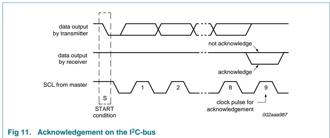
Fig 11. Acknowledgement on the I<sup>2</sup>C-bus
