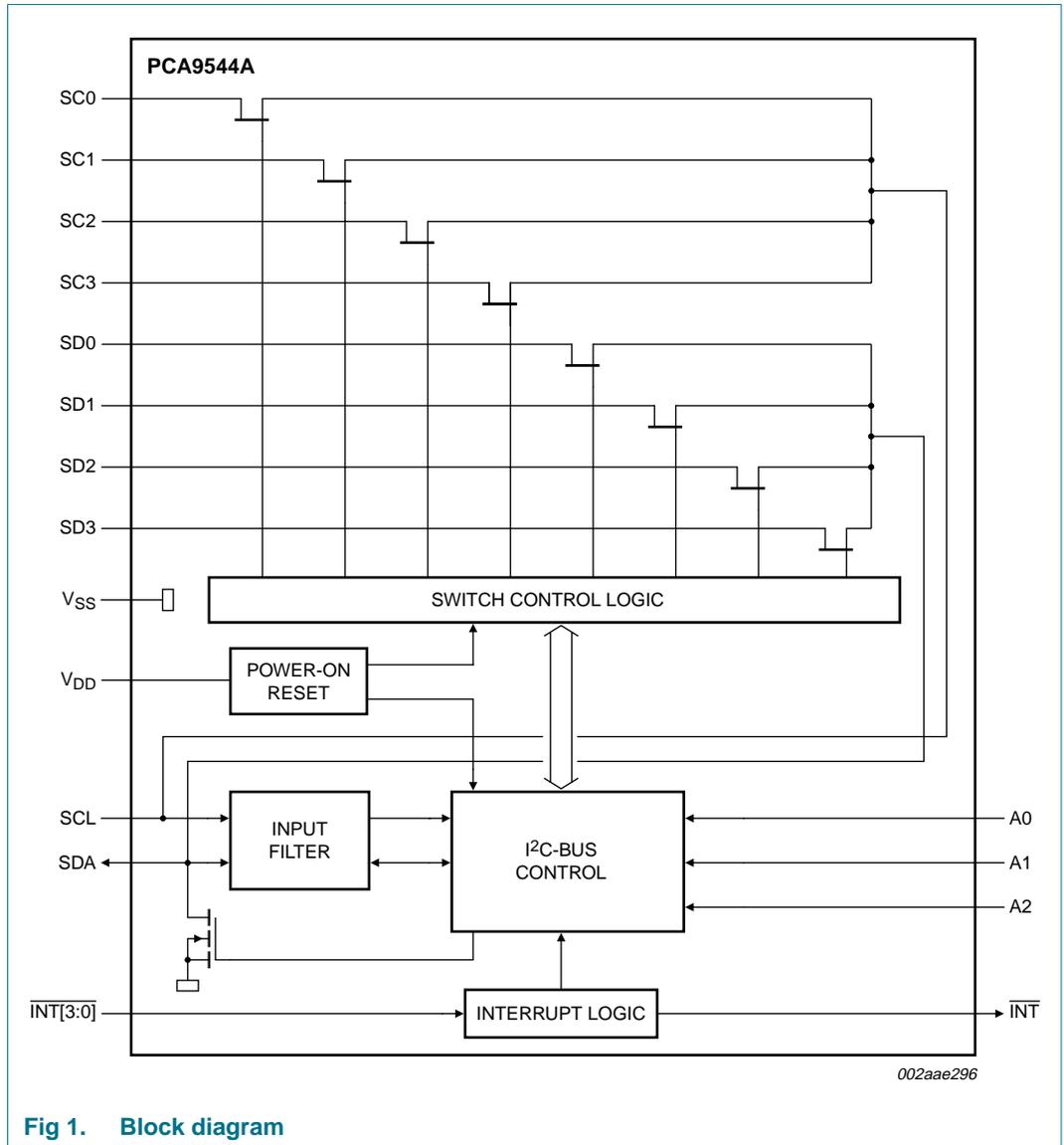
Fig 1. Block diagram
