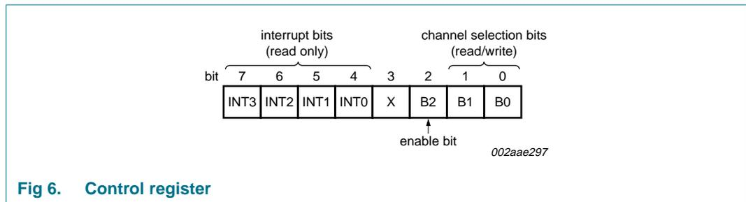
Fig 6. Control register
