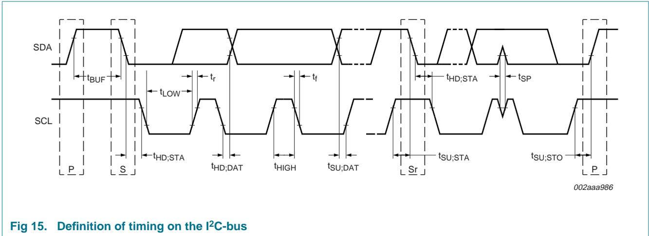
Fig 15. Definition of timing on the I<sup>2</sup>C-bus
