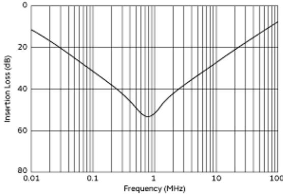
Common Mode Insertion Loss (Typ.)
