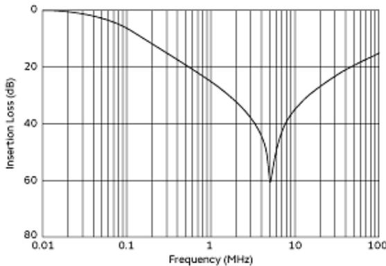
Differential Mode Insertion Loss (Typ.)
