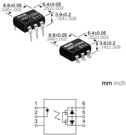
**1. PhotoMOS relay with high response speed, low leakage current and low On resistance**
