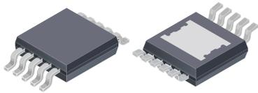
16-pin TSSOP with exposed thermal pad (suffix LP)
