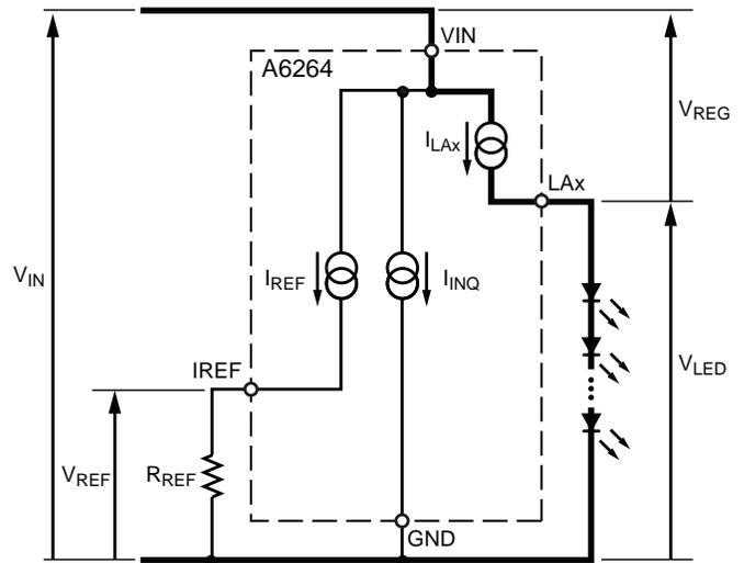
Figure 3. Internal power dissipation sources.
