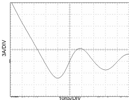
**Figure 22. FDS6994S SyncFET body diode reverse recovery characteristic.**
