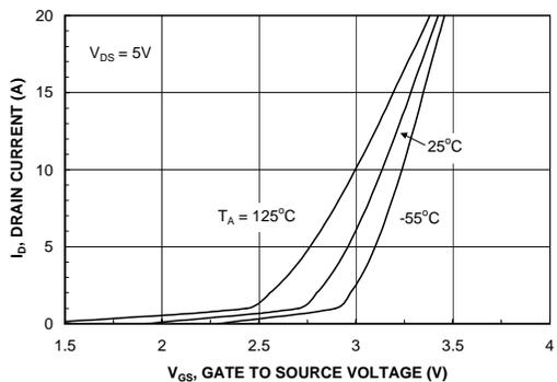
Figure 15. Transfer Characteristics.
