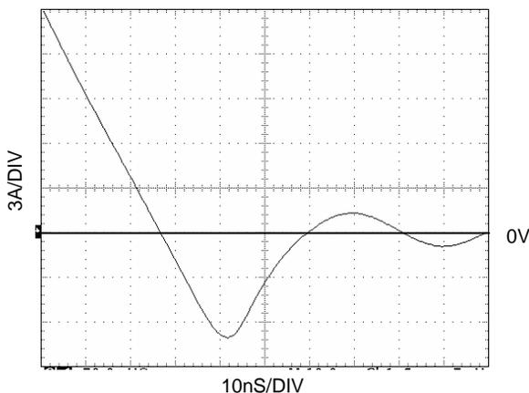
**Figure 23. Non-SyncFET (FDS6690A) body diode reverse recovery characteristic.**
