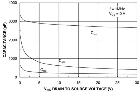
Figure 8. Capacitance Characteristics.
