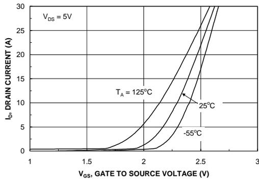
Figure 5. Transfer Characteristics.
