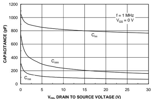
Figure 18. Capacitance Characteristics.
