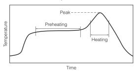
For soldering (Example : Sn/Pb)
