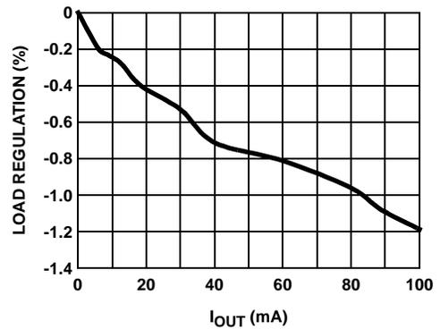
FIGURE 12.  $V_{OFF}$  LOAD REGULATION
