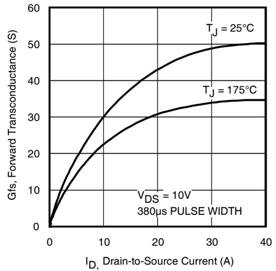
**Fig 4.** Typical Forward Transconductance Vs. Drain Current
